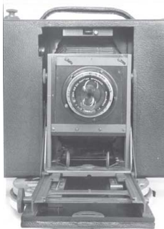
Figure 5. The No. 6 Cirkut Camera, showing the extra sharp Wollensak triple convertible lens.
