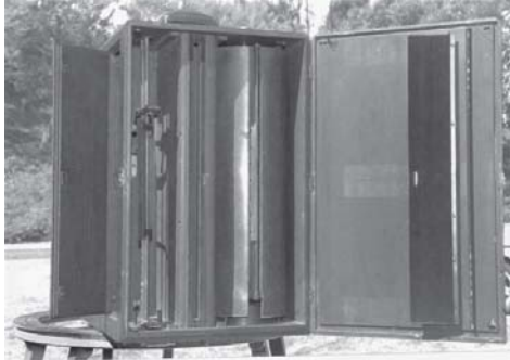
Figure 8. The Century Camera Co. No. 16 camera with open film box.
