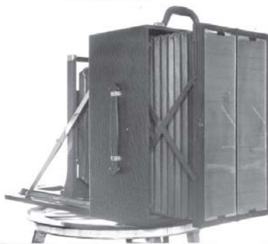
Figure 10. The No. 16 Cirkut with the film box removed with the ground glass extended to focus on the next picture.
