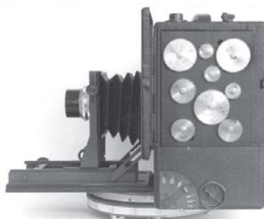
Figure 6. The No. 6 Cirkut open, exposing the nine pinion gears. Notice it is taller than the No. 5 Cirkut shown in Figure 4.
